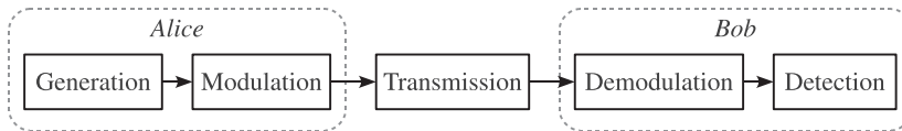
Fig. 5. Diagram of the optical part of a QKD system, where Alice and Bob denote the sender and the receiver, respectively.
